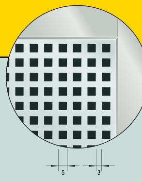
40 mm thick Aluminum frame with perforated sheets. Standard colour - anodized aluminum. Other RAL colours available on request. Standard lifetime of springs - 20.000 cycles (available up to 100.000 cycles).
